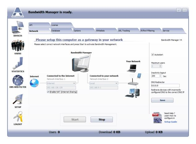
The first step in setting up the Bandwidth Manager is sharing Internet connection. This step is required in order to allow all customers in your network to access the Internet.
