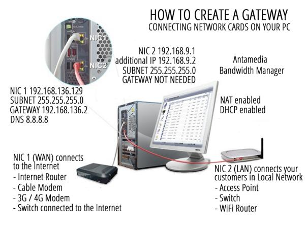
Note that 2 network cards on the Bandwidth Manager server cannot be bridged, the Internal network has to operate in different IP range than External network. Please refer to the diagrams for the example IP settings.
