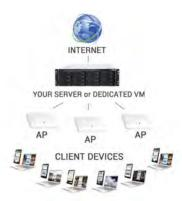
On Premise WiFi System will be deployed on servers hosted in your company, or in a dedicated cloud VMs. It includes Captive portal, AAA Radius, database, Network Controller, Web Filter and HotspotOS for access points.
